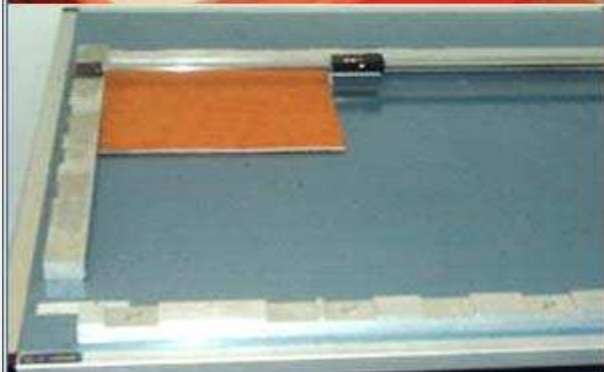
09. Dimensional stability test
